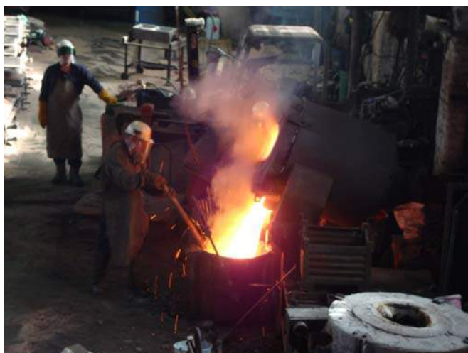
The metal being poured from the furnace prior to pouring into the mould.
